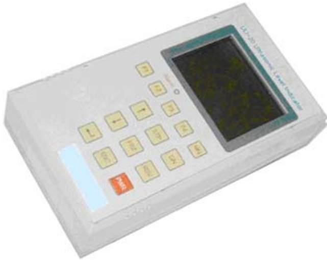
FIG. 5. Manufactured equipment for measuring precursor consumption for field application.
